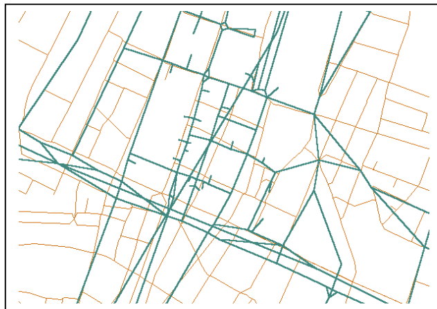
Figure 1. An example of an accurate digital road network model (brown) and an inaccurate road traffic model network model (green).
